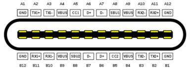
Figure 6: USB Type-C receptacle pinout
