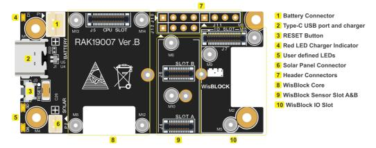
Figure 4: RAK19007 top view components
