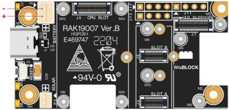
Figure 7: Battery connector pin order
