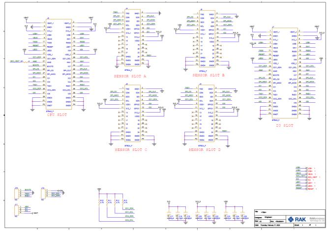
Figure 16: RAK19007 schematic diagram (Slots)
