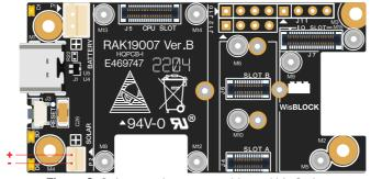
Figure 8: Solar panel connector V+ and V- Order
