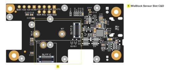
Figure 5: RAK19007 bottom view components
