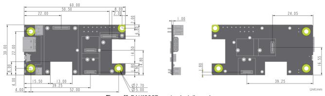
Figure 11: RAK19007 mechanical dimensions
